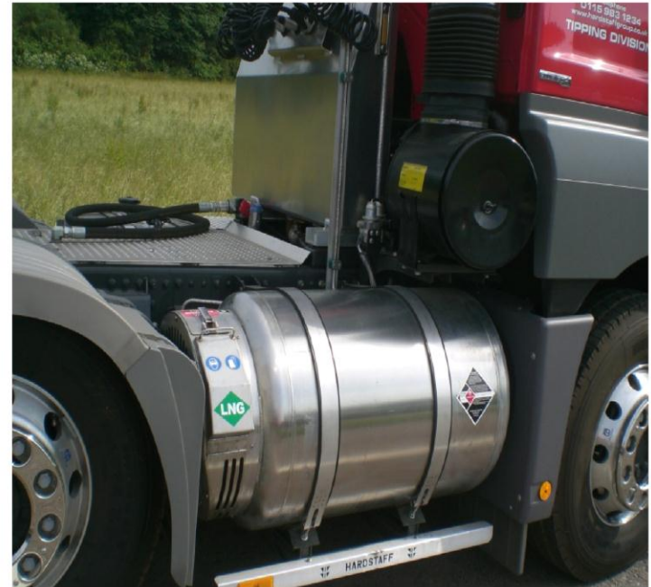
LNG stored in cryogenic tank containment
